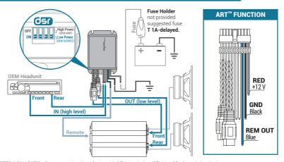
DSR: DOUBLE STEP-DOWN RATIO, allows correct level interfacing with 0EM Headunit or 0EM Amplifier by switch selection.
