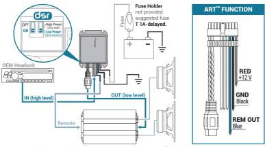
DSR: DOUBLE STEP-DOWN RATIO, allows correct level interfacing with 0EM Headunit or 0EM Amplifier by switch selection.
