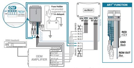
DSR: DOUBLE STEP-DOWN RATIO, allows correct level interfacing with 0EM Headunit or 0EM Amplifier by switch selection.
