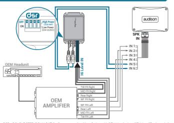
DSR: DOUBLE STEP-DOWN RATIO, allows correct level interfacing with OEM Headunit or OEM Amplifier by switch selection.
