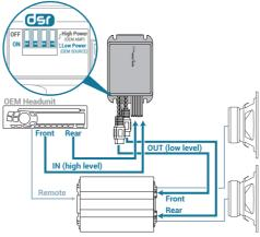
DSR: DOUBLE STEP-DOWN RATIO, allows correct level interfacing with OEM Headunit or OEM Amplifier by switch selection.
